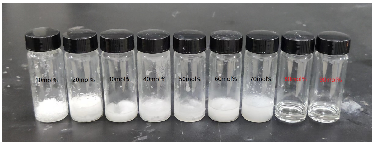
Figure 1. Photographs of BMIMCl/Urea mixtures with different molar fraction at room temperature ( MF_{\text{BMIMCl}} = 10\% \sim 90\% )
