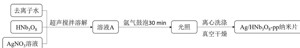
Figure 2. Schematic illustration of \text{Ag}/\text{HNb}_3\text{O}_8\text{-pp} nanosheets photocatalyst synthesis 图 2. \text{Ag}/\text{HNb}_3\text{O}_8\text{-pp} 纳米片光催化剂合成示意图
