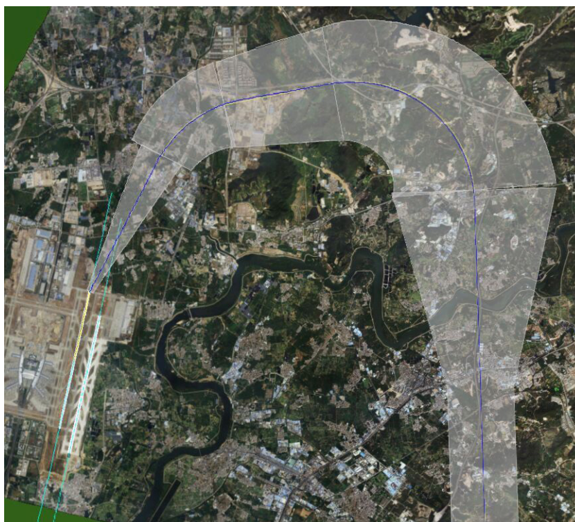
Figure 9. Comparison of takeoff simulation trajectories and design trajectories 图 9. 起飞模拟轨迹与设计轨迹对比
