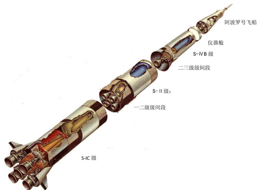
Figure 1. The structure diagram of Saturn V launch vehicle [6]
