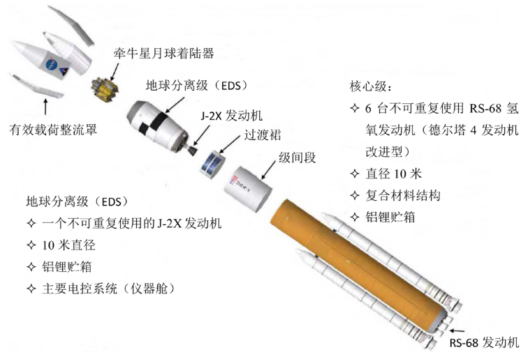
Figure 7. The structure diagram of Ares V launch vehicle [15] 图 7. 战神五号火箭结构图[15]
