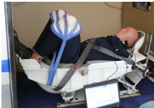
Figure 1. Seat-dummy system in supine position
