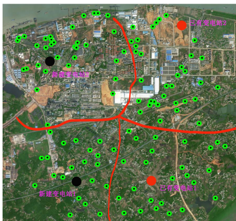
Figure 3. The simulation results of substation planning using density approach 图 3. 密度法初始化变电站规划仿真结果
