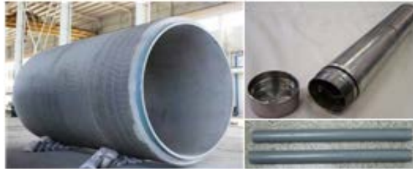
Figure 11. Experimental PCCP and inspection instruments
