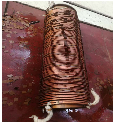
Figure 2. String excitation destabilizing coil 图 2. 串变激磁失稳线圈
