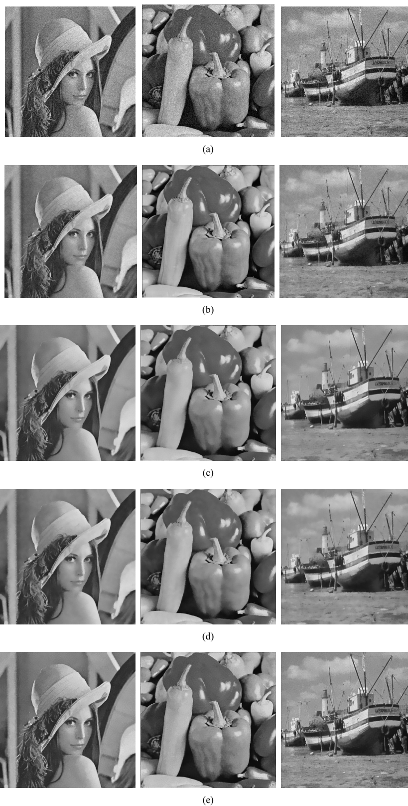
Figure 2. Comparison of restoration results for different standard test images with \sigma_n = 20 of Gaussian white noise: (a) Noisy images; (b) Bilateral filtering; (c) Non-local means; (d) Order statistical based bilateral filtering; (e) Proposed algorithm 图 2. 对高斯白噪声 \sigma_n = 20 的标准测试图像 Lena、Peppers、Boat 的滤波结果对比: (a) 噪声图像; (b) 双边滤波; (c) 非局域均值滤波; (d) 次序统计量相似度双边滤波; (e) 文中算法
