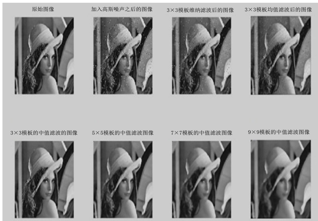
Figure 1. Resulted images under different operating 图 1. 滤波效果对比图
