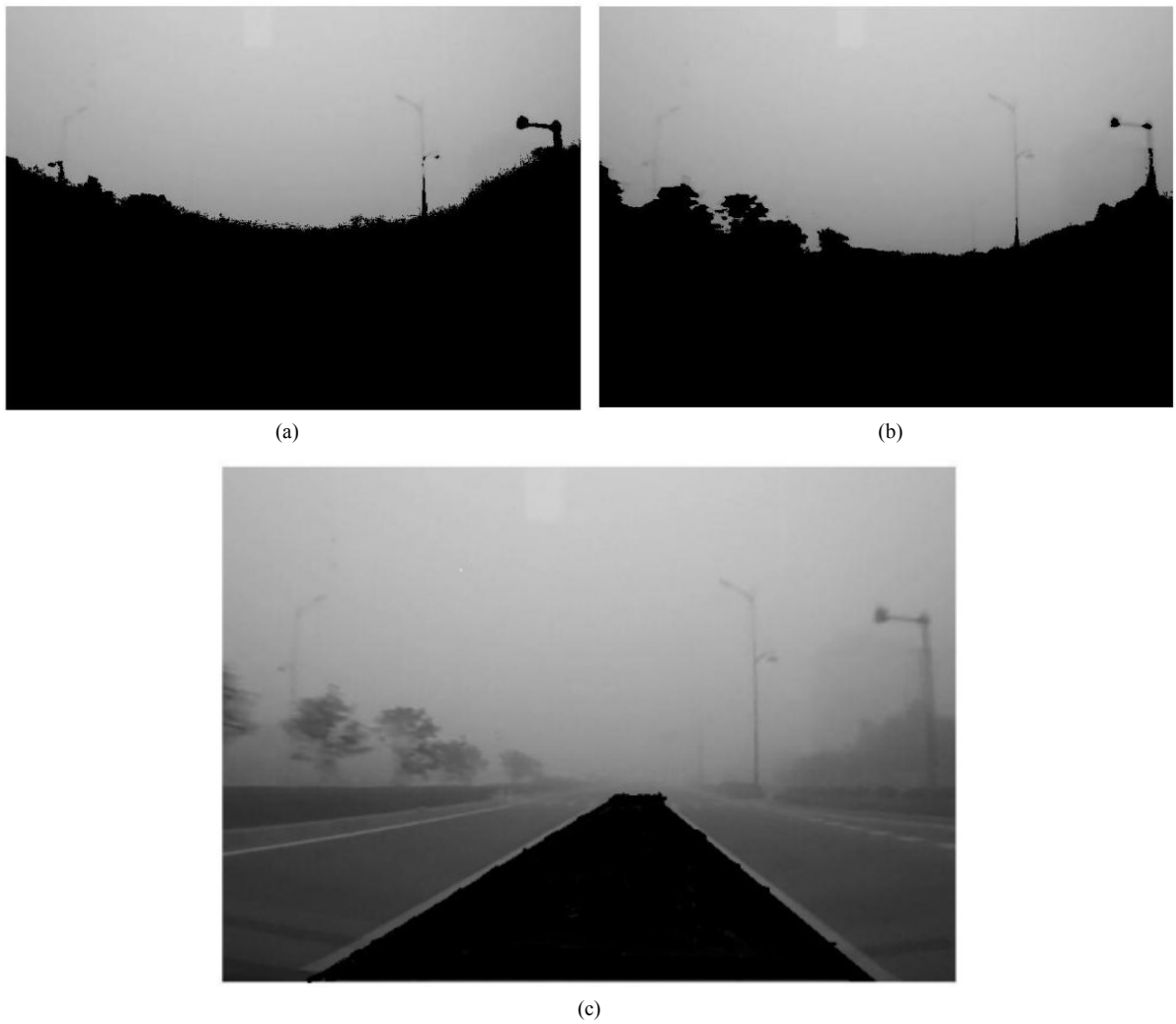
Figure 5. Comparison of different region segmentation results. (a) Otsu threshold segmentation; (b) Iterative threshold segmentation; (c) Custom region growing 图 5. 多种区域分割结果比较。(a) Otsu 阈值分割; (b) 迭代式阈值分割; (c) 自定义区域增长
