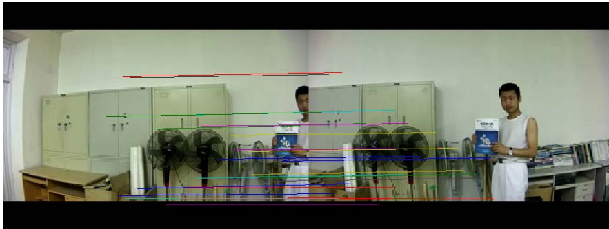
Figure 8. The original purification of SURF feature points matching 图 8. 原始 SURF 特征点提纯匹配
