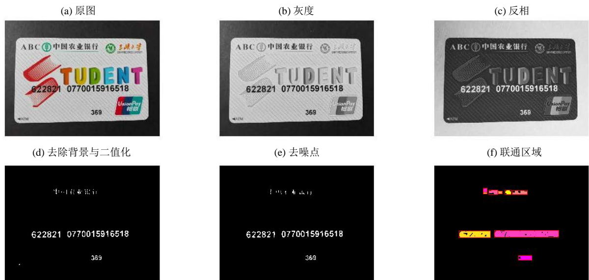
Figure 2. The bank card number automatic identification process map 图 2. 农行卡号自动识别过程图
