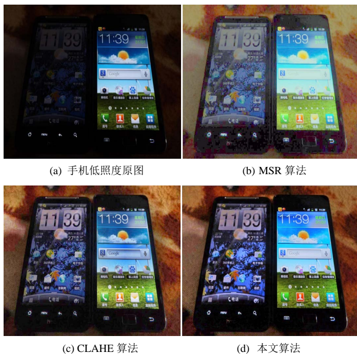
Figure 2. Comparison of different algorithms for mobile phone low illuminance image enhancement
