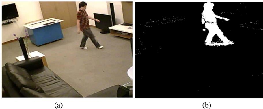
**Figure 2.** Motion targets obtained by Vibe algorithm. (a) Original image of moving human body; (b) Images of human body detected by Vibe algorithm
