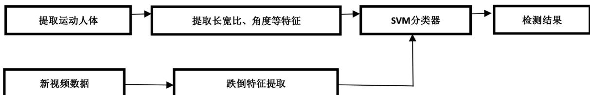
Figure 4. Fall detection process of Multi-feature fusion and SVM
