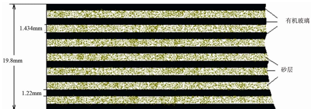
Figure 2. The model of the sandstone and mudstone thin interbed
