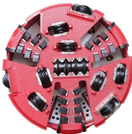
Figure 2. The arrangement plan of tool pan and cutters
