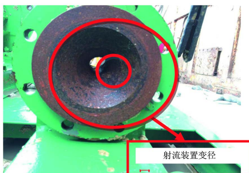
Figure 2. The jet slurry mixing device
