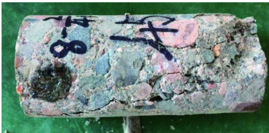
Figure 3. The test result of core compressive and failure test 图 3. 岩心抗压破坏试验结果图
