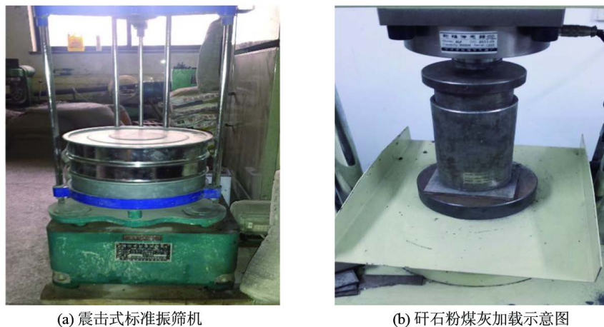
Figure 2. The schematic diagram of specimen loading equipment 图 2. 试件加载设备示意图
