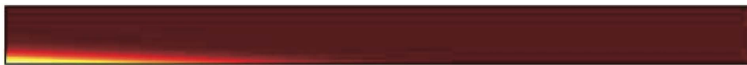
Figure 2. The distribution of temperature field of single point steam injection from heel
