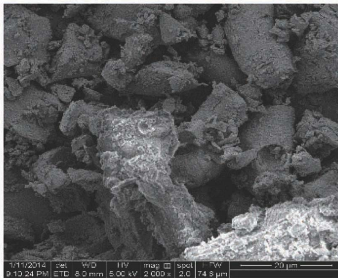
Figure 1. Scanning electron microscope diagram of scale in Well J1 图 1. J1 井垢扫描电镜图
