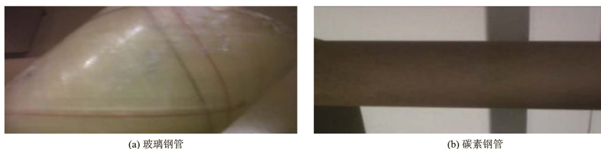
Figure 1. The comparison of corrosion resistance of steel pipe 图 1. 不同种类钢管的耐腐蚀能力对比
