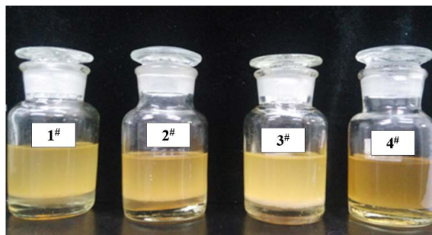
Figure 5. Broken milk pictures of emulsion with different \text{NaCl} concentrations after high temperature aging 图 5. 高温老化后不同 \text{NaCl} 浓度乳液破乳图片
