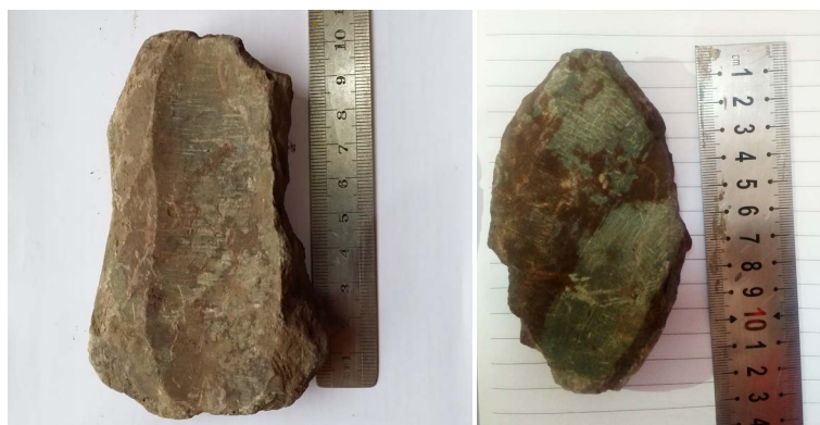
Figure 1. Gaomiao 33-4HF and Gaomiao 33-9HF well fall-block 图 1. 高庙 33-4HF 与高庙 33-9HF 井掉块
