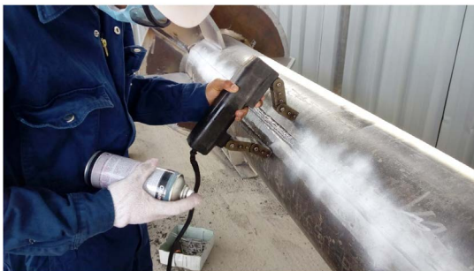
Figure 9. Magnetic particle testing 图 9. 磁粉检测
