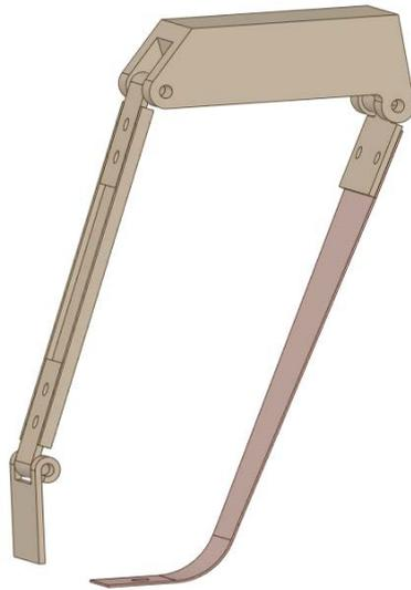
Figure 7. Schematic diagram of the improved spring support structure
