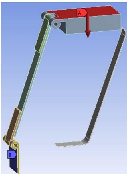
Figure 3. Schematic diagram of the loading and fixing method of the probe mechanism
