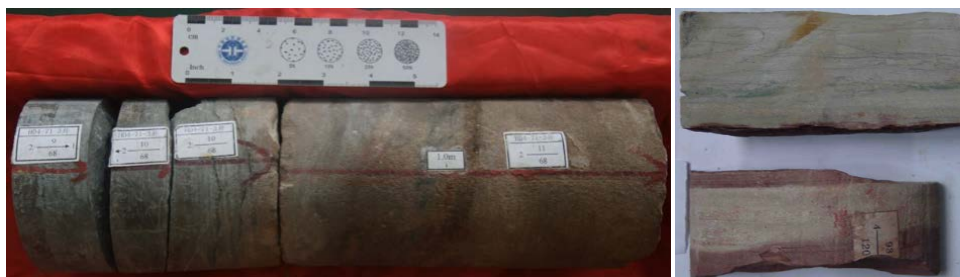
Figure 2. Unconformity (left: top erosion unconformity; right: bottom top super-unconformity) 图 2. 不整合面(左: 顶部削蚀不整合面, 右: 底部上超不整合面)
