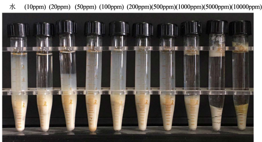
Figure 1. Anti-swelling effect of PASC 8 clay stabilizer
