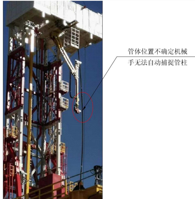
Figure 2. Due to the uncertain position of the bent pipe body, the robotic arm is unable to automatically capture the physical image of the pipe column
