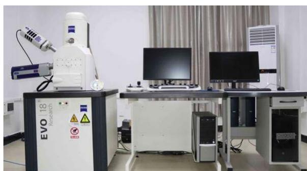
**Figure 3.** Scanning electron microscope
