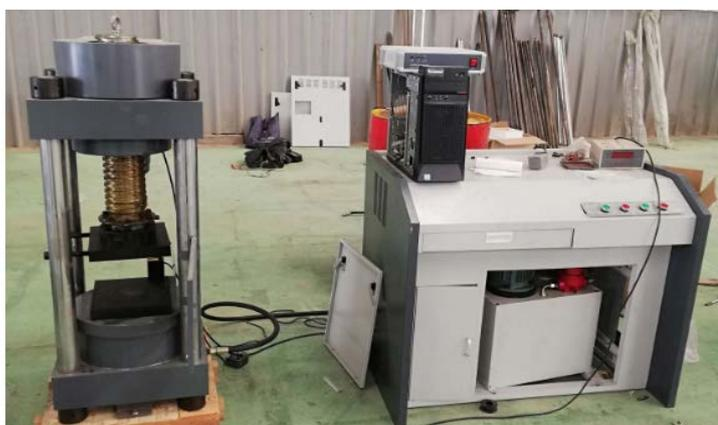
Figure 7. Brazilian splitting test instrument
