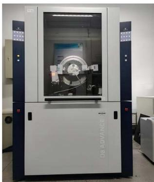
**Figure 1.** X-ray Diffractometer
