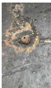
Figure 1. Macroscopic morphology of perforation in weld 图 1. 焊缝处穿孔宏观形貌图
