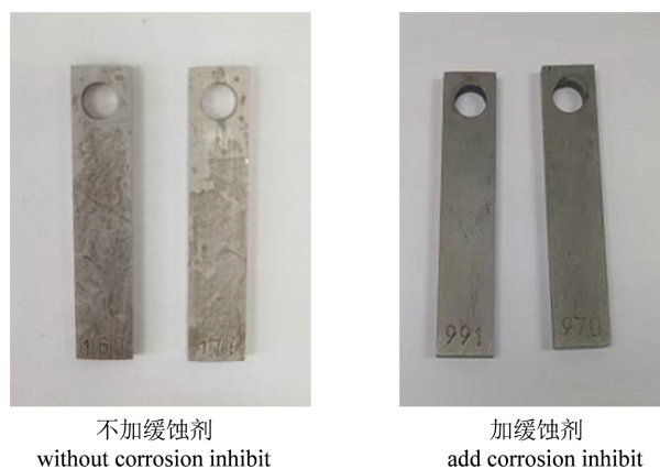
Figure 5. Comparison of steel sheet corrosion
