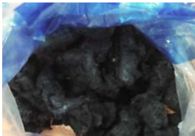
Figure 2. Organic scale samples attached to the downhole string 图 2. 井下管柱上附着的有机垢样
