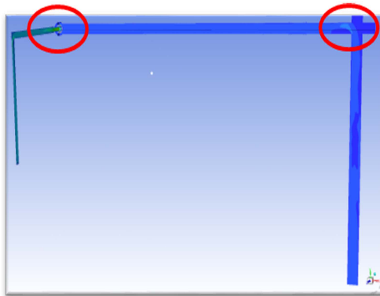
Figure 4. Maximum thickness thinning position of wellhead wall 图 4. 井口壁厚最大减薄位置
