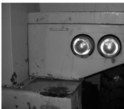
Figure 4. Improvement of mine vehicle lighting
