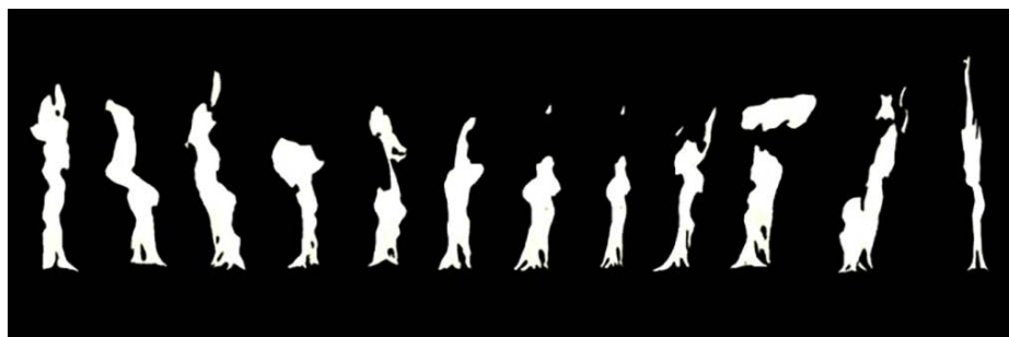
Figure 8. Flame swing state at wind speed of 1.6 m/s (1 s interval)
