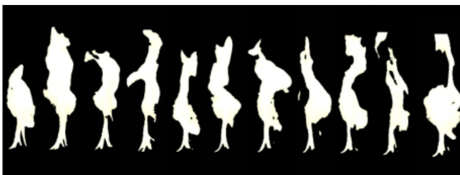
Figure 6. 0.8 m/s transverse air (interval 1/10s)
