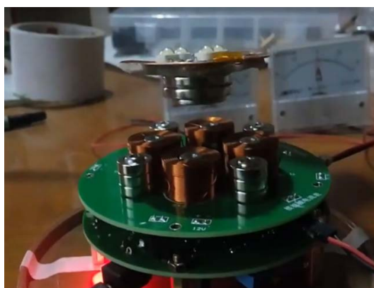
Figure 19. Magnetic levitation device to achieve stable suspension 图 19. 磁悬浮装置实现稳定悬浮
