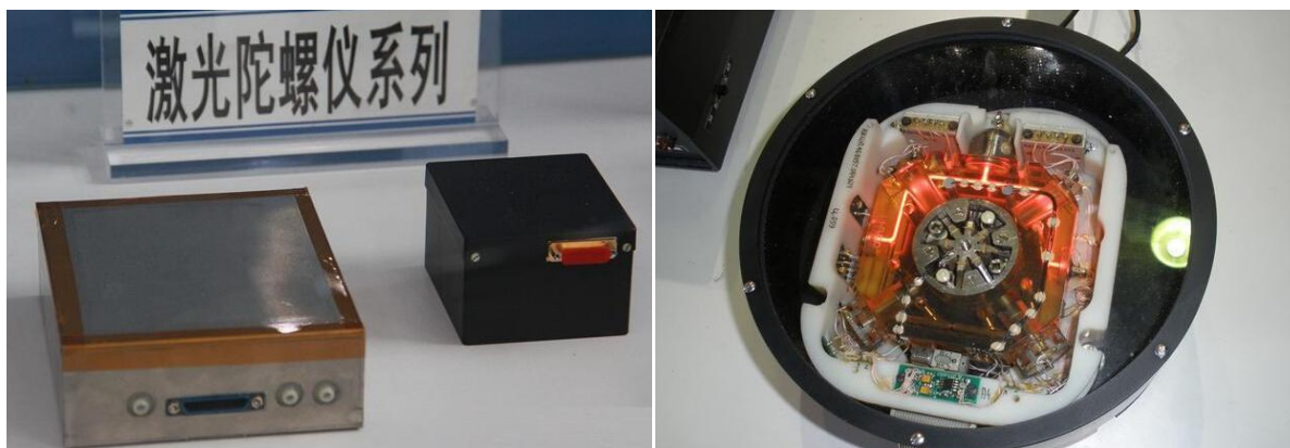
Figure 1. Laser gyroscope and its internal structure 图 1. 激光陀螺仪及内部构造
