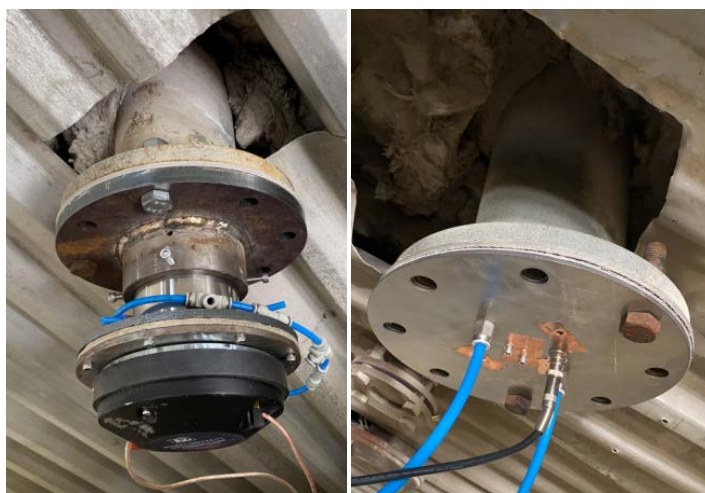
Figure 4. Mounting structure of speaker and microphone 图 4. 扬声器及传声器安装结构
