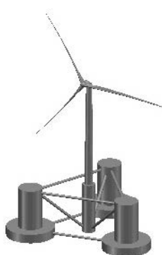
Figure 3. SNL13.2 MW semi-submersible floating wind turbine diagram 图 3. SNL13.2 MW 半潜式浮式风机示意图
