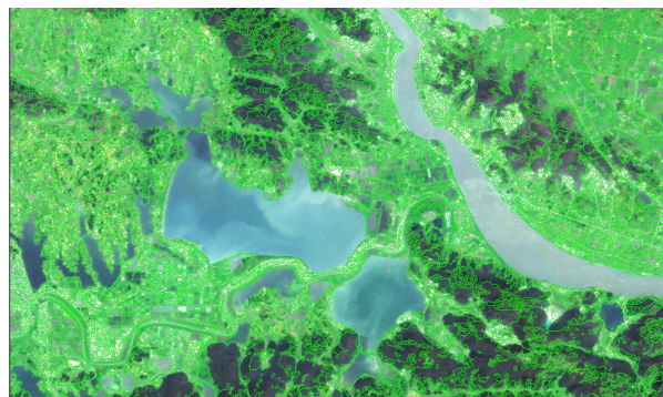
Figure 7. Band classify as a pixels based on the distance between each wave 图 7. 根据波段间距离分类将相近程度小于阈值的像元化为一类
