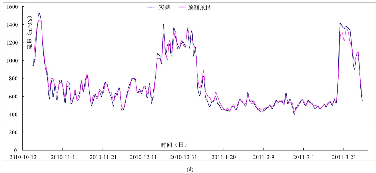
Figure 2. Comparison of simulated and predicted low flow hydrograph in Guigang hydrologic station: (a) The simulated and predicted low flow hydrograph from October 1974 to March 1975; (b) The simulated and predicted low flow hydrograph from October 1985 to March 1986; (c) The simulated and predicted low flow hydrograph from October 2002 to March 2003; (d) The simulated and predicted low flow hydrograph from October 2010 to March 2011
