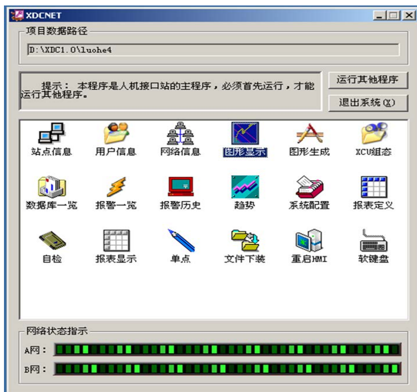
Figure 4. Software interface of water plant based on DCS 图 4. 基于 DCS 架构的自来水厂智能控制系统软件界面
