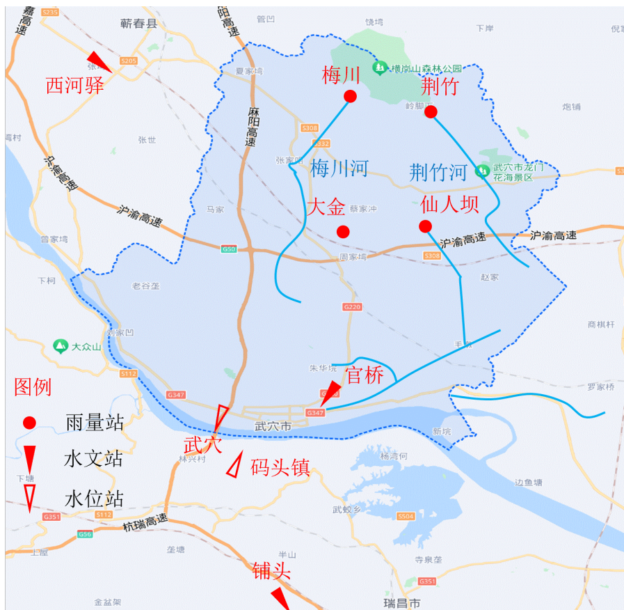
Figure 1. Study regional river system and hydrographic station network distribution diagram 图 1. 研究区域河流水系及水文站网分布示意图
