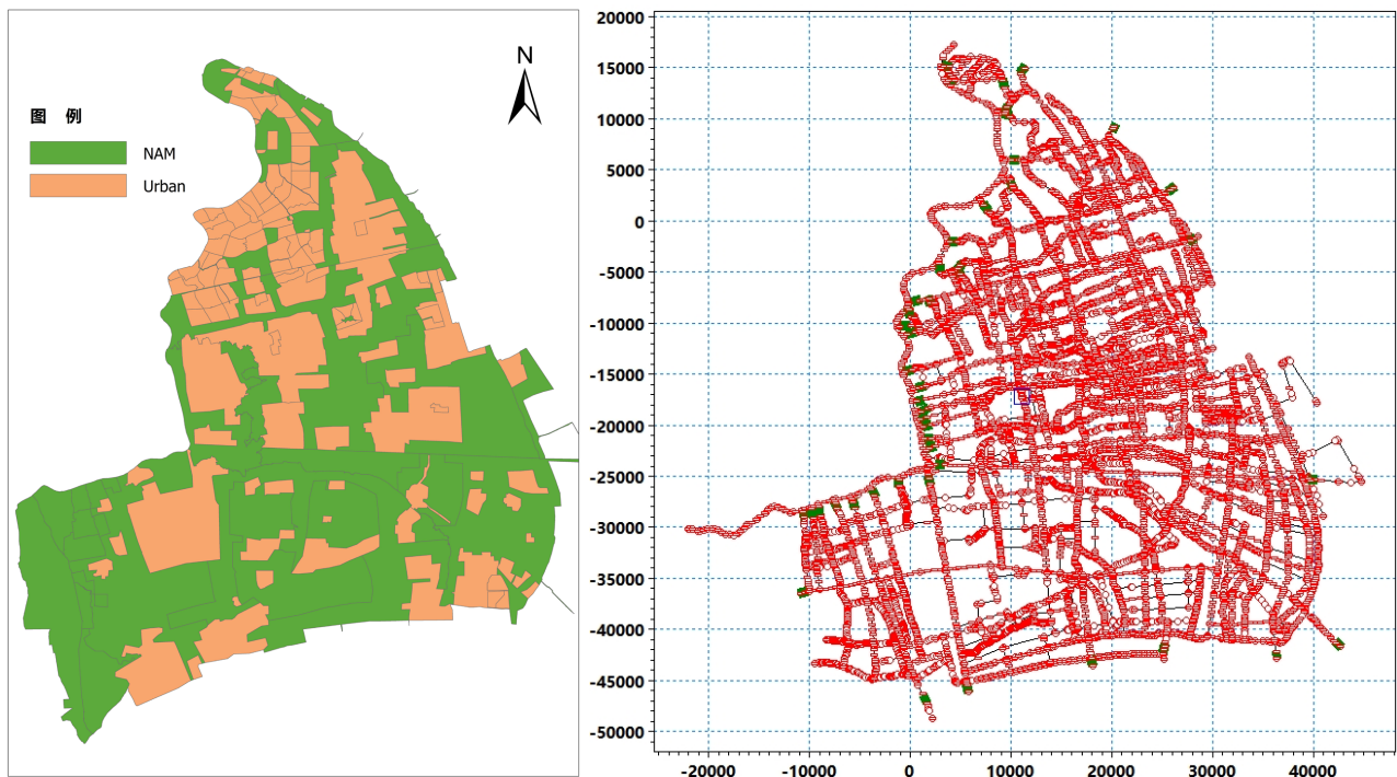
Figure 3. Hydrological and hydrodynamic model hydrological zoning and river network overview map of Pudong water conservancy area
