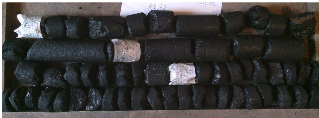
Figure 2. Z_3 after injection of 40 - 44.5 32 - 40 m hole in m by fetching coal core diagram (2013-YL-296) 图 2. Z_3 孔 32~40 m 注水后在 40~44.5 m 所取煤芯图(2013-YL-296)
