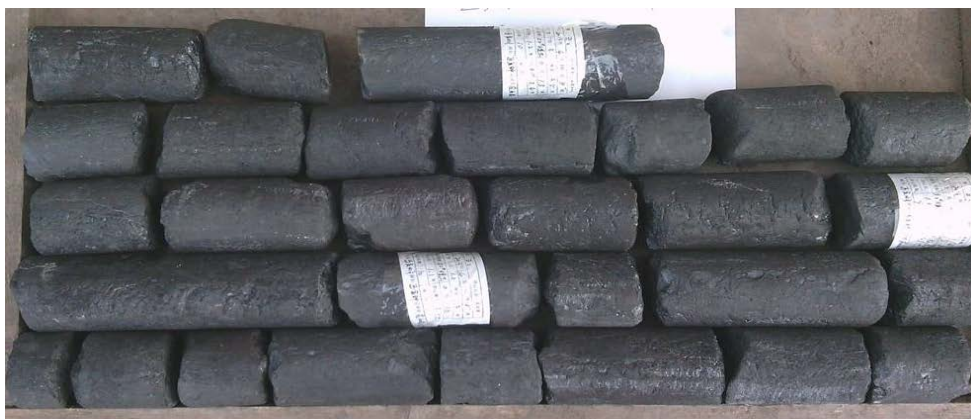
Figure 1. Before injection hole by fetching coal core graph Z_3 图 1. 注水前 Z_3 孔所取煤芯图
