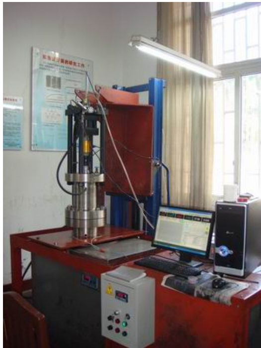
Figure 2. Triaxial stress thermal-hydro-mechanical coal containing gas permeameter 图 2. 含瓦斯煤热流固耦合三轴伺服渗流实验装置
