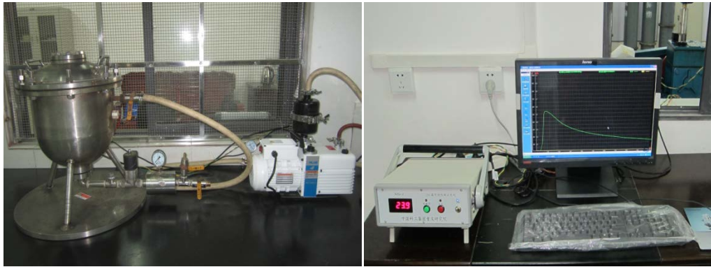
Figure 1. 20 L dust explosion characteristics test system 图 1. 20 L 粉尘爆炸特性测试系统
