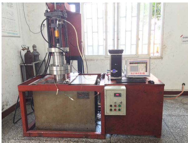
Figure 1. Tri-axial stress thermal-hydrological-mechanical Coal Gas Permeameter
