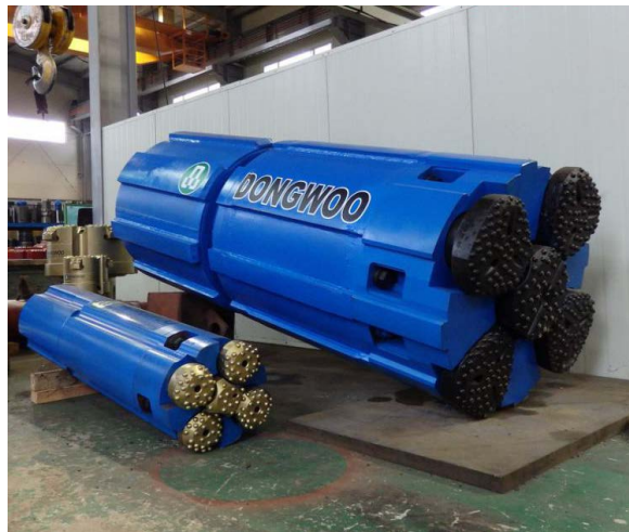
Figure 8. Cluster pneumatic reverse circulation DTH hammer 图 8. 集束式气动反循环潜孔锤
